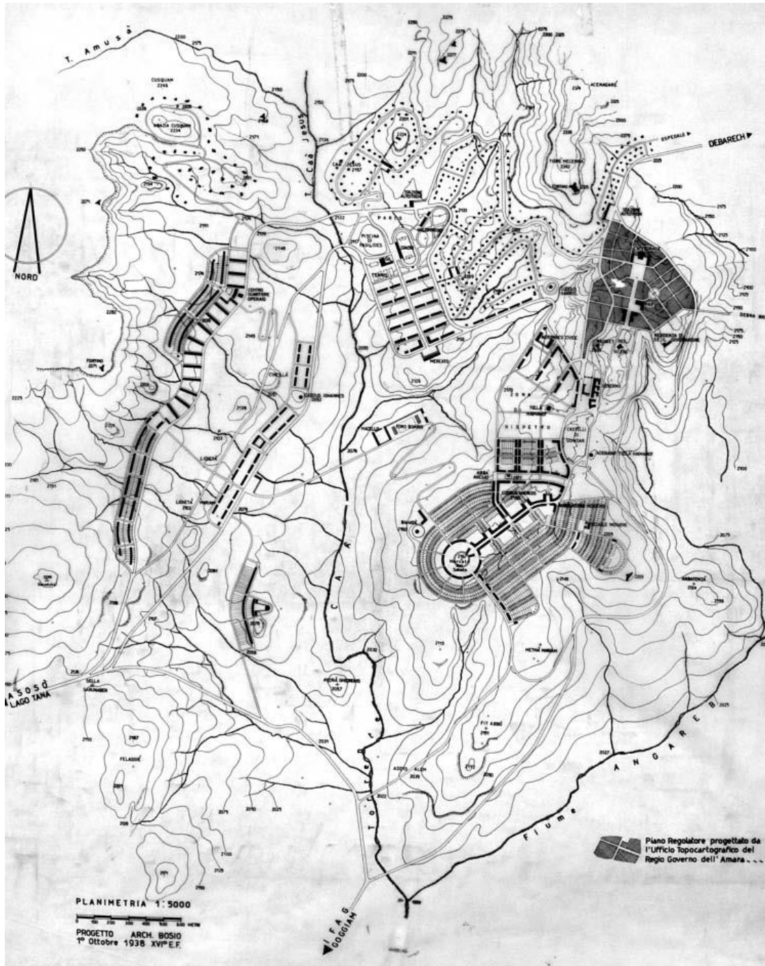
Figure 55: Gherardo Bosio and Ufficio Topografico del Regio Governo dell' Amara (shaded section), Master plan for Gondar, 1 October 1938, AEGB, 1:5000 scale, 25 metre contour interval, north consistent with orientation.
