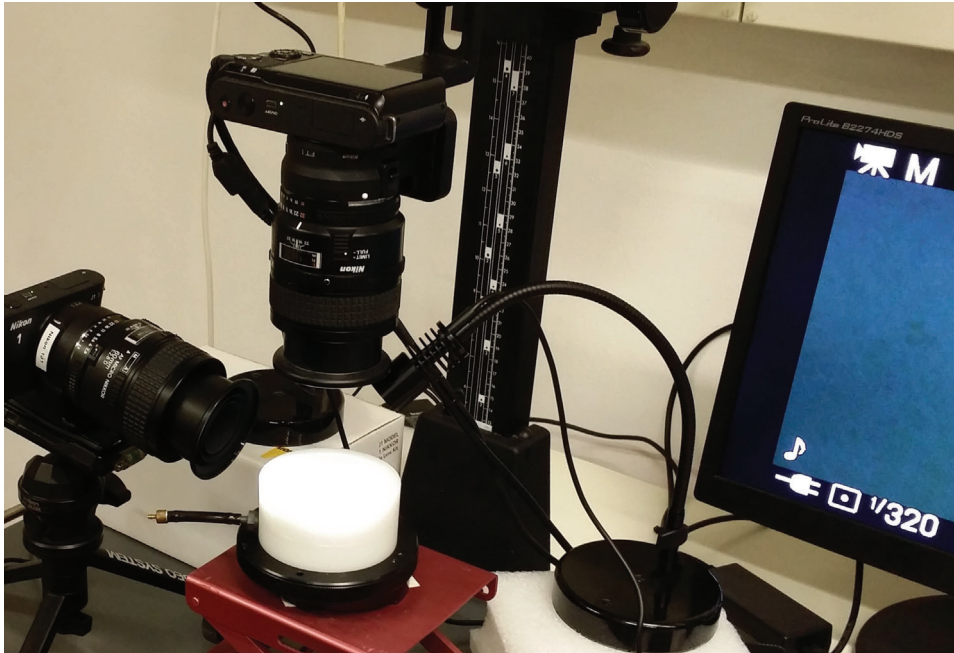
Figure 4.8: Custom mite recording setup with two cameras, macro lenses, and a platform.
